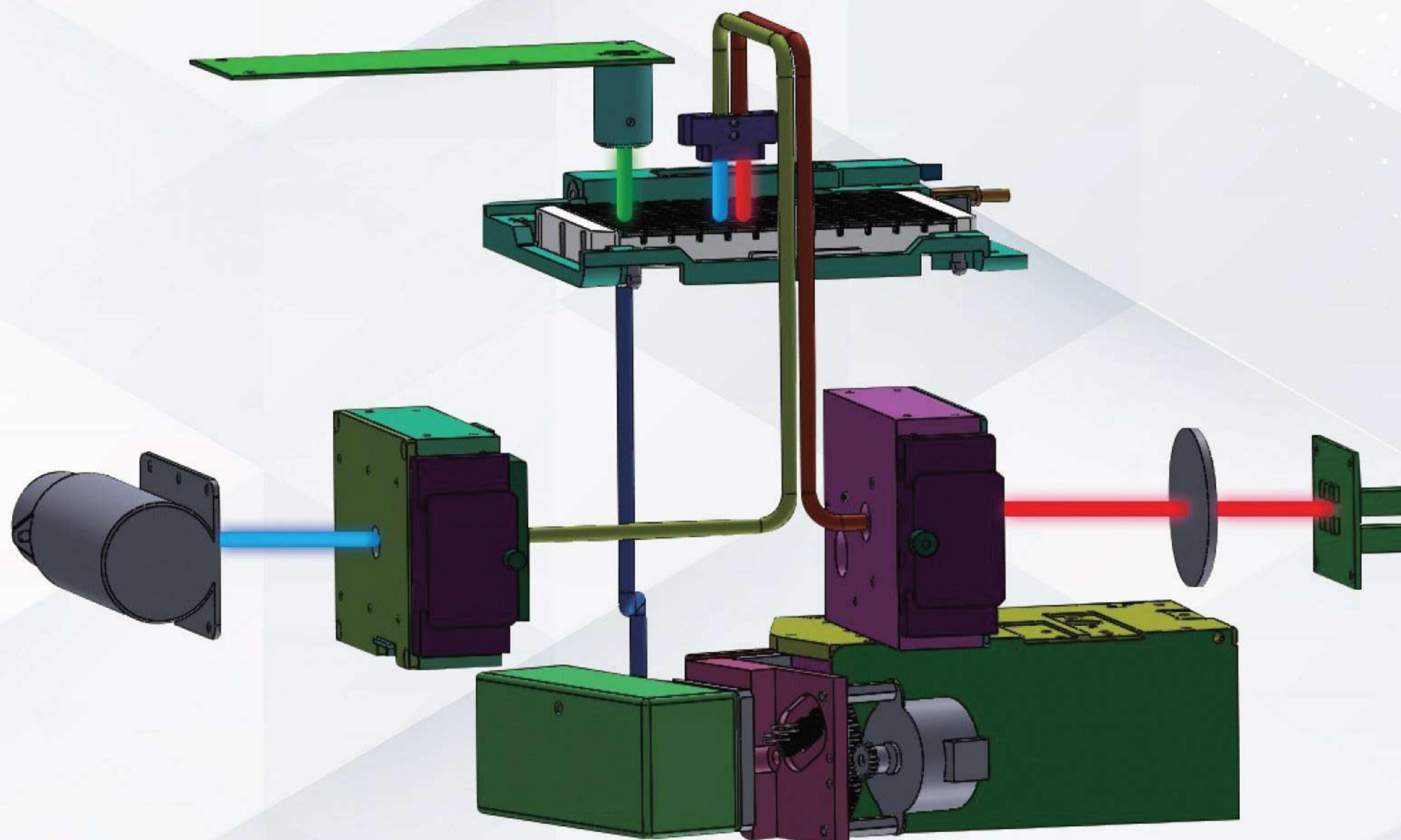
INNO-S™ has three main detecting functions. Since INNO-S™ is a monochromator-based microplate spectrophotometer for the absorbance measurements, it requires zero filters and allows you to measure from 200 to 999 nm freely at your choice of 1nm increment. Also Xenon lamps in absorbance will serve the instrument semi-permanent life time which brings the comfortable experiences to the users since the lamps do not need to be replaced such as halogen lamps.
